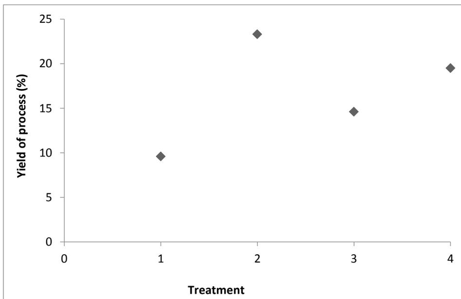
**Figure 3:** Yield results for the Spray Drying process, where 1 represents temperature 100°C, 2 represents temperature 105°C, 3 represents temperature 110°C and 4 represents 130°C.
